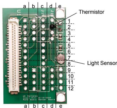
◀ **NOTE:** If you have downloaded the pdf schematic of the Rene basic sensor board from UC Berkeley, you will see that the A/D channels appear in reverse order. This is due to a difference in wiring between the original Rene Mote and the MICA/MICA2 family of motes.
