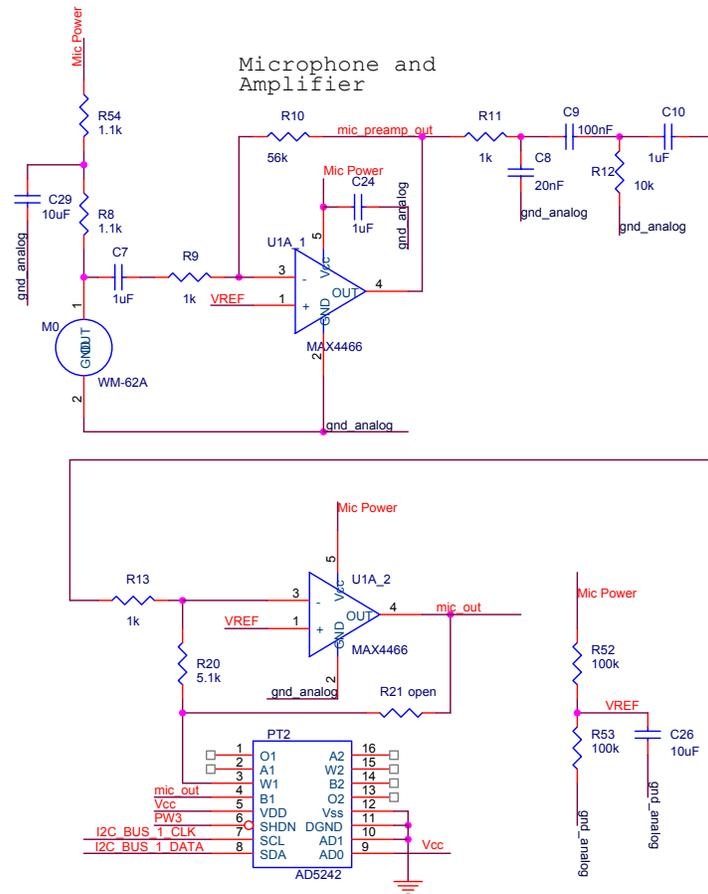
Figure 3-5. MTS310CA Schematic of Microphone and Amplifier.
