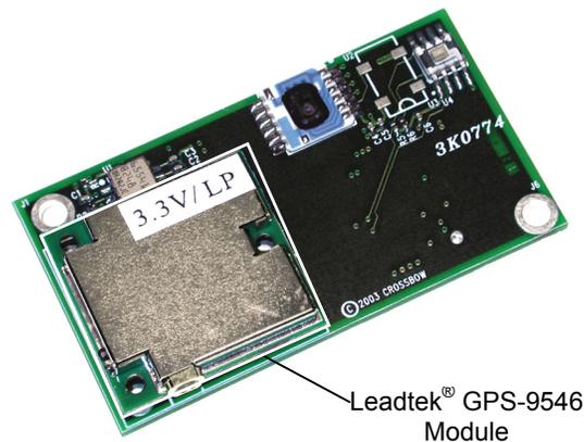
**Figure 4-1.** Photo of MTS420CA. The MTS400CA does not have the GPS module (highlighted by the box).
