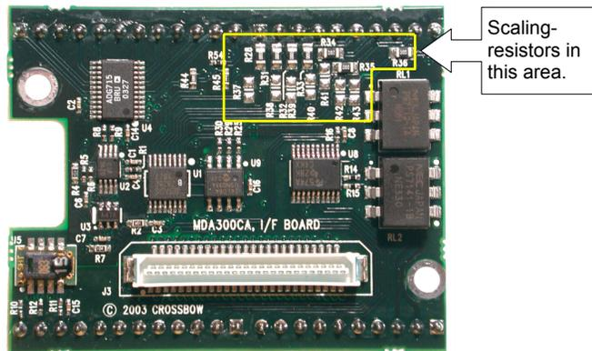
**Figure 6-3.** Photo of backside of the MDA300CA.
