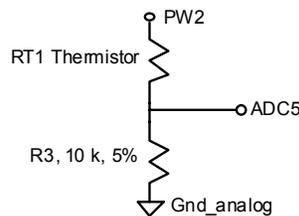
**Figure 2-1. Thermistor Schematic.**
