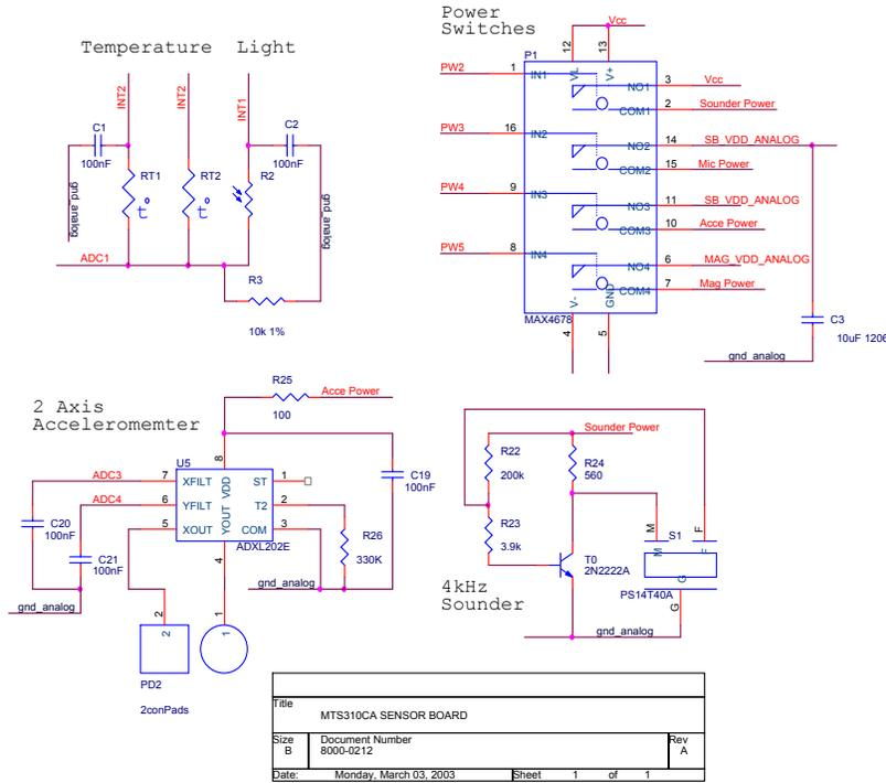
Figure 3-3. MTS310CA Schematics of Accelerometer, Sounder, Temperature and Light Sensors, and Power Switches
